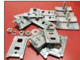
Complete set of clips to install moldings on both sides of car.
