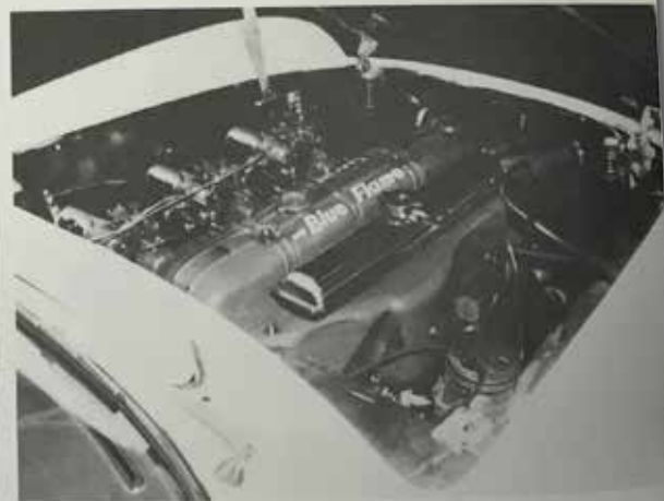
Powering the majority of the first-year Corvettes was the new Blue Flame Six, most fitted with three Carter side-draft carburetors. However, a few of these cars were reportedly built using small GMC truck engines. Because of the low hood profile, the radiator expansion tank was located on the block, adjacent to the rocker arm cover. The spark plugs and distributor are enclosed by a special shroud. When installed in the Corvettes, the Blue Flame engine had its compression raised to 8.0:1, which resulted in 150 horsepower at 4200 RPM.
