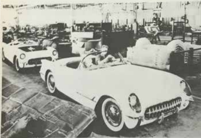
Coming off the Flint assembly line is the first of the 300 Corvettes produced in Michigan this year. In January, 1954, production would officially be switched to the St. Louis plant. Directly behind the car can be seen stacks of rear underbody units of the unique reinforced fiberglass bodies. Although called production models, these first-year Corvettes were essentially hand-crafted semi-production automobiles, and differed from each other in many small ways — as can be witnessed by the Bel Air wheel covers on the first car.
