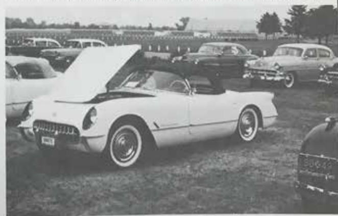
protruding exhaust tips, sunken and glassed license plate, and lack of full bumpers. It was also the first production car to use a body of reinforced fiberglass. Entering production in June, 1953, the car was designated the Model 2934 and given a base price of $3,513.
